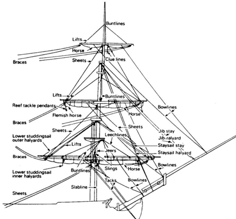
FIGURE 3. Main rigging on a ship's foremast. Source: Kemp (1976).
